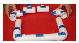
Glue Part 25 and Part 27 together using Part 26. Make sure they are both even and at the same angle. This can be done by placing them on a flat surface.
