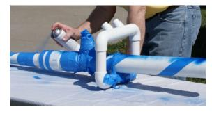
tape. For painting multiple colors, tape off the machine for one color at a time. Allow plenty of drying time between colors.
