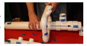
Place the pipe strap 9/1/2 inches behind the 3x3x2 inch reducing tee. It is your option to screw the pipe strap onto the 3 inch PVC pipe so that it will be extra secure.
