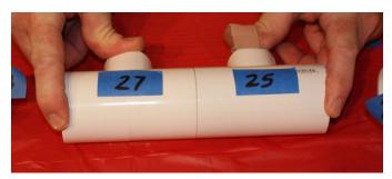
Dry fit the upper armature together by inserting Part 27 into Part 28 and Part 24 into Part 25. You will want to glue them so that Part 27 and Part 25 are at a 45 degree angle. This does not have to be precise, but you can measure the angle if you like.
