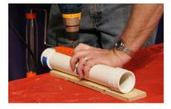
Pivot the paint roller so that spinning roller is <u>4" above</u> the projected air stream, keeping slot and paint roller parallel to each other. Attach a second screw in the handle and pipe to secure this pitch.
