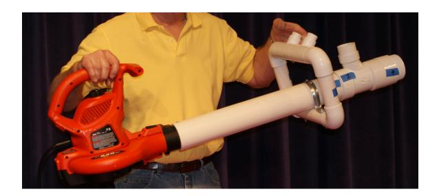
**NOTE:** For illustration purposes only, we use a Black & Decker blower assembly that produces 240 mph airflow. You may use any blower assembly that suits your purposes. The primary requirements are that the blower have a 3" round output, to fit into the 3" PVC pipe and deliver at least a 200 mph output airflow.
