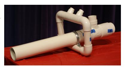
Attach the Poof Cannon to the blower motor. Slide the blower into the pipe. To create as snug a fit as possible, you may want to leave an attachment on the blower or wrap the nozzle with duct tape. Secure with a screw.
