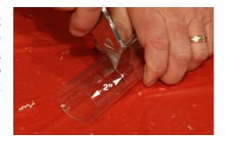
• Glue sparingly to join them. Do not apply glue around the inside lip of the PVC. Apply glue to the clear plastic. This will prevent glue drops from squeezing out into the path of the ping pong balls flowing through the pipe. Apply glue around the outside of one end of the clear plastic and insert it into the coupling. Glue lightly around the other end of the clear plastic and insert it into the second coupling.
