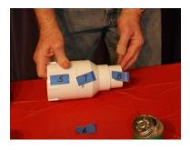
• Glue Part 9 to Part 8. Note: Parts 7 & 9 fit tightly together.
