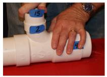
• Part 16 fits onto Part 15 as a dry fit and is not to be glued. It needs to be removable so the crepe paper used with "The Crepe Paper Flame Thrower" can flow in. Cut Part 16 as you did Part 12, using Part 14 to secure the cap as you cut it. Crepe paper normally is 1 ¾" wide. The slot needs to be the right size so that the crape paper can freely flow through the tube.
