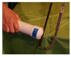
remove the cut piece. Sandpaper the rough edges to remove all burrs. **Make sure all the shavings are out**, remove the cap and smooth the inside of the cut.
