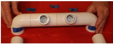
Unhook one dry fitting, glue it, unhook the other dry fitting and glue it. Take care to maintain a 45 degree angle.
