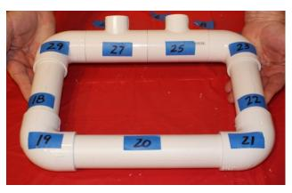
Glue 30 and 31 into the handle assembly. Keep a rag handy to wipe off excess glue. Both should be inserted to the same depth.
