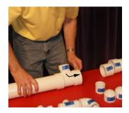
Apply glue to the other side of Part 2. Slide Part 3 into Part 2.
