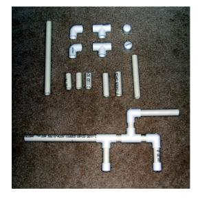
Smooth all rough edges from cut PVC. Wash all of the parts with hot, soapy water. Dry and lay out your pieces in the manner shown below. Firmly insert each piece into the next one. You may glue or seal the tubes together, **BUT this will greatly limit your ability to clean or unclog the Marshmallow Gun.**
