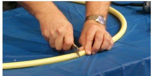
While holding the Hula Hoop at the appropriate angle, 45°, drill a guide hole through the tee and into the Hula Hoop. Insert a screw.
